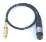
This cable is used to adapt the level, impedance and balance of digital XLR outputs, allowing the PAS-8 outputs to be connected to unbalanced coaxial inputs. Levels, balancing and impedance are converted to standard SPDIF values without any format conversion taking place. Please note that the receiving device needs to be able to process the transmitted format. The cable is usable for sample rates up to 192 kHz. Available lengths: 0.5 m, 1.0 m, 2.0 m and 3.5 m.
